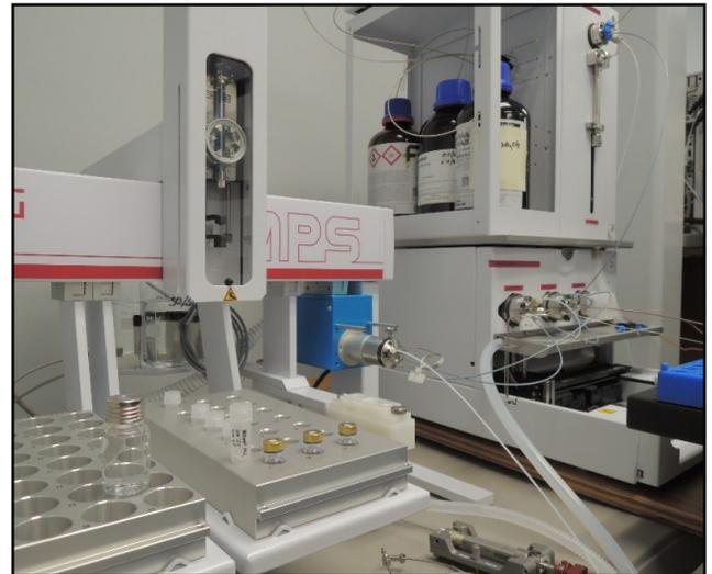
Figure 3- Gerstel Automated Multi-Purpose Sampling and SPE System
