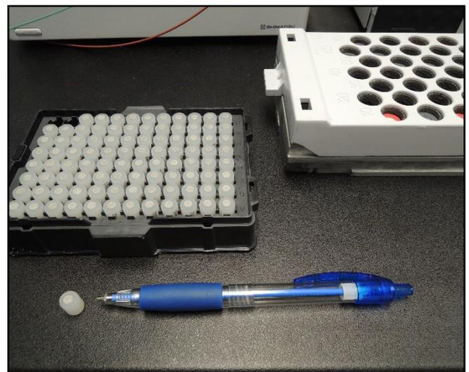
Figure 4 - Customized Solid Phase Extraction Cartridge
