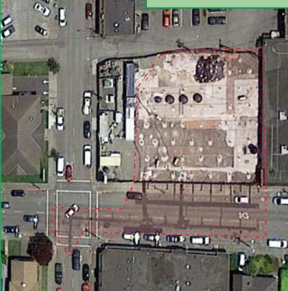
Contamination source area extended beneath a busy public road where subsurface utilities, including AT&T's main West coast fiber-optic and communication conduit are buried within the treatment volume , requiring special design considerations to minimize traffic impairments, thermal impacts, and electro-magnetic interference (EMI) to the buried utilities.
