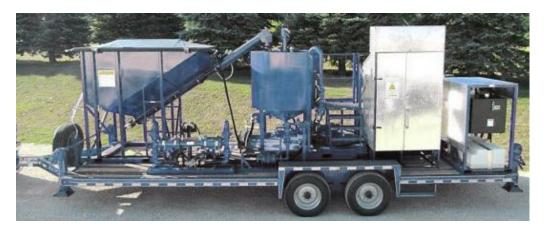
This fully automated mobile mixing trailer can mix and inject slurry with accuracy to the nearest pound. Digital load cells provide accurate measure units at all times. The super sack loading system eliminates the need for manual handling of injection materials, ensuring that your project is completed safely and efficiently.
