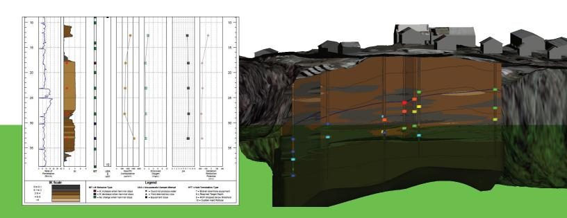
Real-time hydrostratigraphic profiling with discrete depth sampling, without withdrawing the tool between samples, allows for efficient high-resolution groundwater investigation. In the example report log on the left, the IK allowed the field technician to identify and sample a sand unit between two clay units that served as a major contaminant transport pathway. On the right is an example of a cross section modeling a Waterloo<sup>APS</sup> data set.
